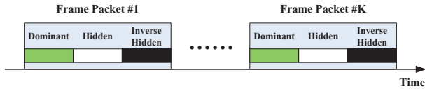
Figure 2: Frame packets contain a set of images to be displayed rapidly in sequence. In our study, frame packets contained three images each: Dominant Image, Hidden Image and Inverse Hidden Image.
